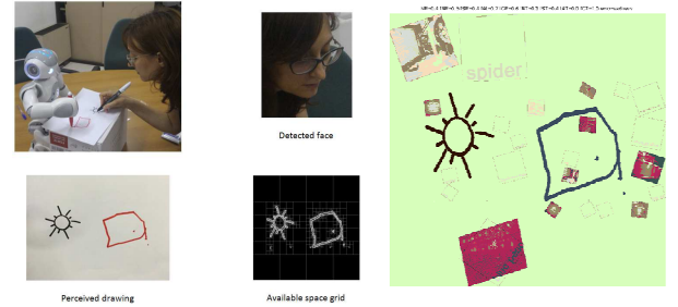
Fig. 2. An example of simple social interaction to perform a drawing collaborative task. The robot verbally interacts with the user, detects a face, uses data from a social app to propose a digital collage.
